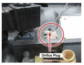
For the unload solenoid you can have 2 types of configurations, one which uses the orifice plate or one that uses the orifice plug. If you are using infinite capacity unloading(pulsing) you would leave these restrictions in place to slow down the unloading. If you are set up for step unloading(on/off) these restrictions should have been removed. Replace the existing solenoid with the new solenoid and 2 gaskets for the orifice plate or 1 gasket for the orifice plug.
